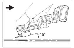
Turn the tool on and then apply the wheel or disc to the workpiece.
