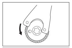
**NOTE:** Ezynut can be loosened by hand as long as the arrow points the notch. Otherwise a lock nut wrench is required to loosen it. Insert one pin of the wrench into a hole and turn Ezynut counterclockwise.
