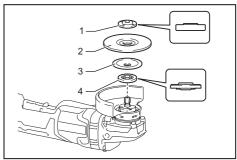
Lock nut 2. Flex wheel 3. Back up pad 4. Inner flange
