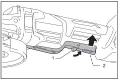
1. Lock-off lever 2. Switch lever
