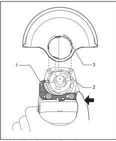
1. Lock lever 2. Notch 3. Protrusion
