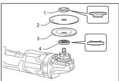
Sanding lock nut 2. Abrasive disc 3. Rubber pad
